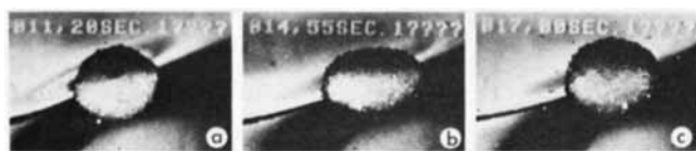
Figure 10. Periodic extension and compression of particle cluster in simple shear flow ( \lambda = 0 ). The volume fraction of particles is 0.5. The same fluid as the bulk medium is used to make the suspension from which the cluster is formed causing the surface tension between the cluster and the bulk to be zero. The cluster thus behaves as a drop with zero surface tension but of higher viscosity than the surrounding medium, initially spherical (Figure 10a), first extended (Figure 10b), then compressed back to its spherical shape (Figure 10c).
